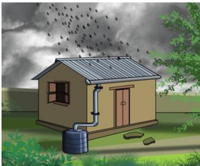
Figure 7.4 Rain water harvesting.
